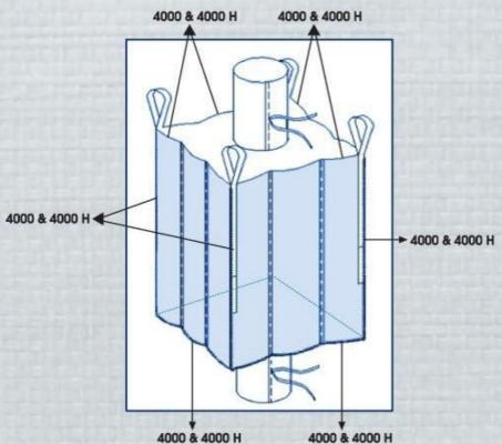
The 4000 series machines are designed for Big Bag producers to sew overlock and safety stitches simultaneously. They possess superior characteristics as well as important modifications to sew today's more difficult Big Bags more efficiently compared to similar machines.
